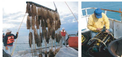
During the TB DBL-152 response V-SOSs were initially used to find submerged oil, however, their results when oiled were not quantifiable enough to initiate diver recovery operations. Since the oil from the TB DBL-152 was denser than seawater, Remotely Operated Vehicles were key to finding areas with recoverable amounts of oil.
