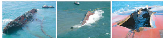
In November 2005 the Tank Barge DBL-152 had initial damage from hitting hurricane debris, then started to take on water and capsized. Total volume spilled estimated at 2 million gallons.
