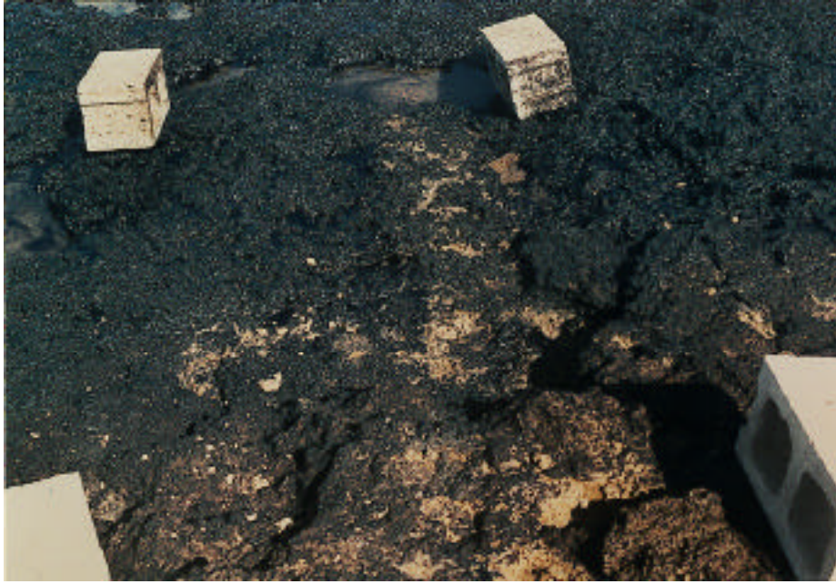
Figure 20A. Plot for high-pressure, hot-water washing alone. The concrete blocks define the corners of the test plot. On the left, washing was conducted with water up to 500 psi and 140°F. Note that very little oil was removed. On the right, washing was conducted with water up to 1,000 psi and 175°F. At this pressure, parts of the rock began to chip off.
