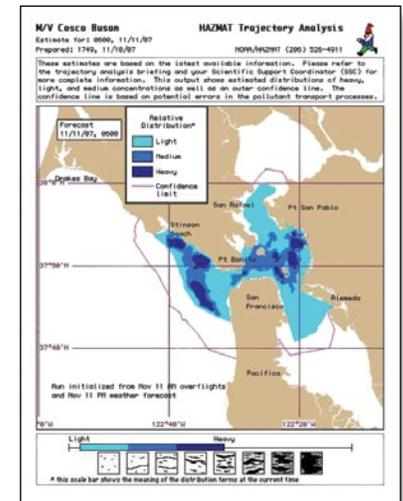
GNOME trajectory output for the M/V Cosco Busan oil spill.
