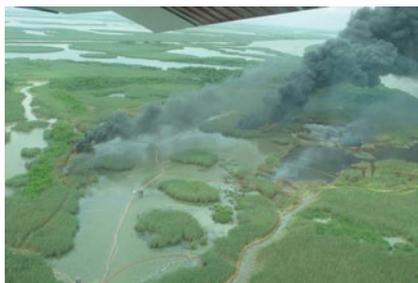
*In situ burn conducted as part of the response to the Octave Header Bulkline spill near Venice, LA, May 2013.*
