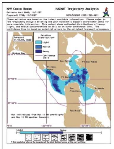
GNOME trajectory output for the M/V Cosco Busan oil spill.
