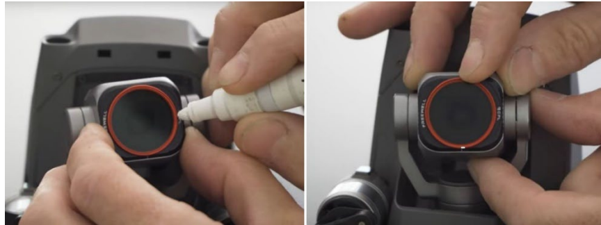
Figure 8. Marking and setting a circular polarizing filter with a mark for setting the horizontal blocking position. Credit: John Daws.
