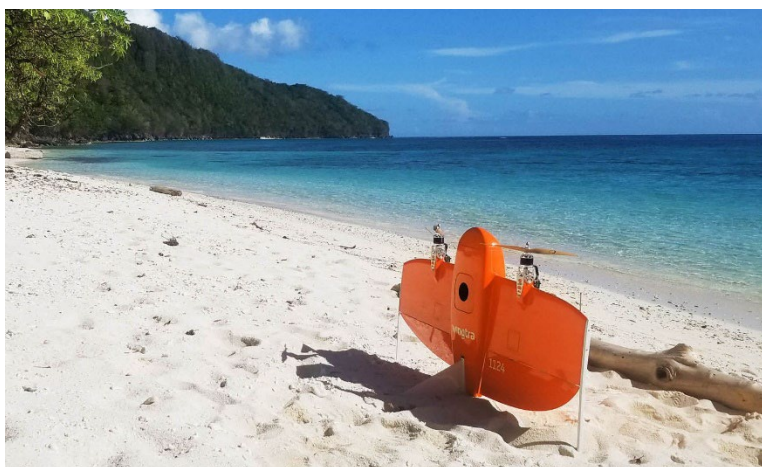
Figure 1. The WingtraOne has vertical takeoff and landing (VTOL) and has been used for Shoreline Cleanup Assessment Technique (SCAT) operations in Australia. Credit: Wingtra.
