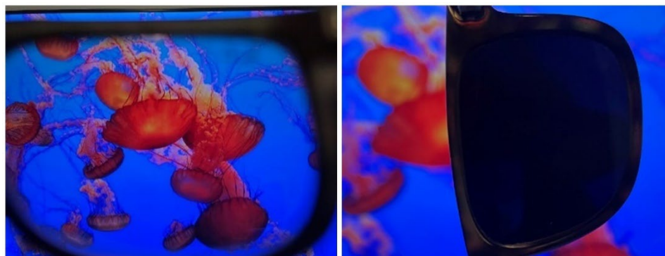
Figure 7. Testing for vertically polarized light. Credit: RPI.
