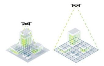
Flying a second pattern that covers the same area at a different altitude (usually 20% higher) may improve mosaic georeferencing accuracy. Processing software is required for producing orthomosaics and processing time increases greatly with an increase in the number of photos used. The most common processing software packages are listed in Appendix B.
